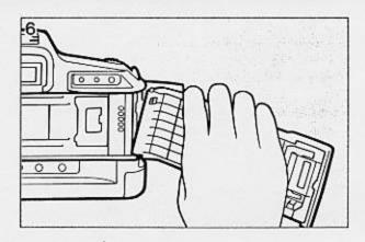
Be sure that there is no film in the camera before attaching the Data Memory Back 90. Otherwise, the film will be exposed when the regular camera back is opened.
